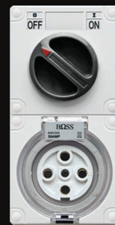
B56C550 50A 500V 5 Round Pins, Triple Poles Switch
